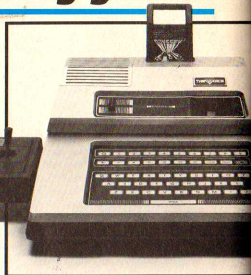
The Voice from Odyssey: The plug-in module has its own speaker.
