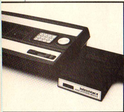
Mattel's voice-synthesis module: no need for separate AC adaptor.
