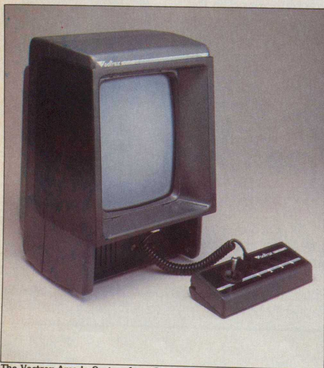
The Vectrex Arcade System from General Consumer Electronics uses a nine-inch black-and-white monitor to offer high-quality visuals.
