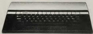
The 1400XL comes with 64K and a built-in modem and speech synthesizer. Will it replace the 1200?
