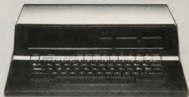
The 1450XL is Atari's second digression into the business market. The new computer carries an on-board dual-density, double-sided disk.
