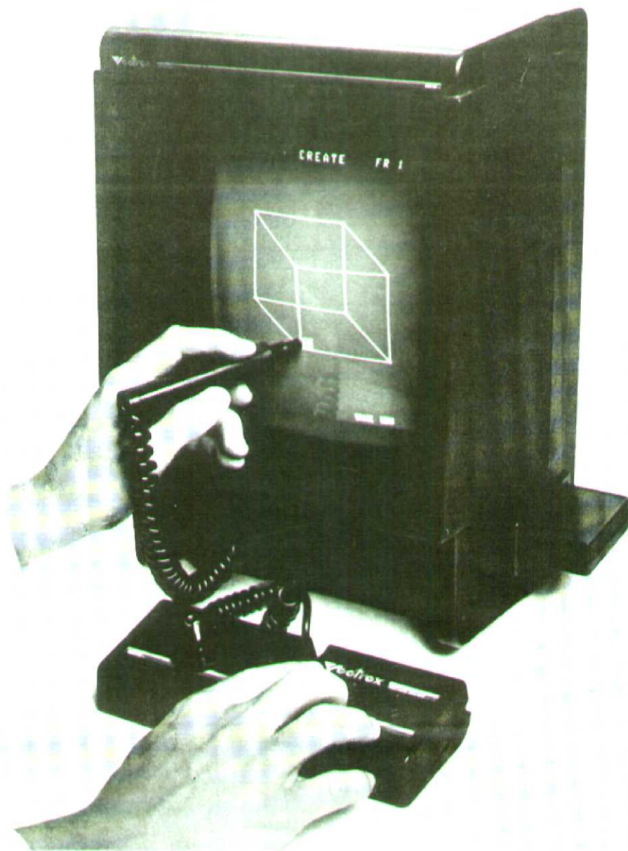
When used in conjunction with the ART MASTER , ANIMATION , MAIL PLANE or MELODY MASTER cartridges, GCE's new Vectrex Light Pen enables users to draw their own pictures or cartoons, play music or study geography.
