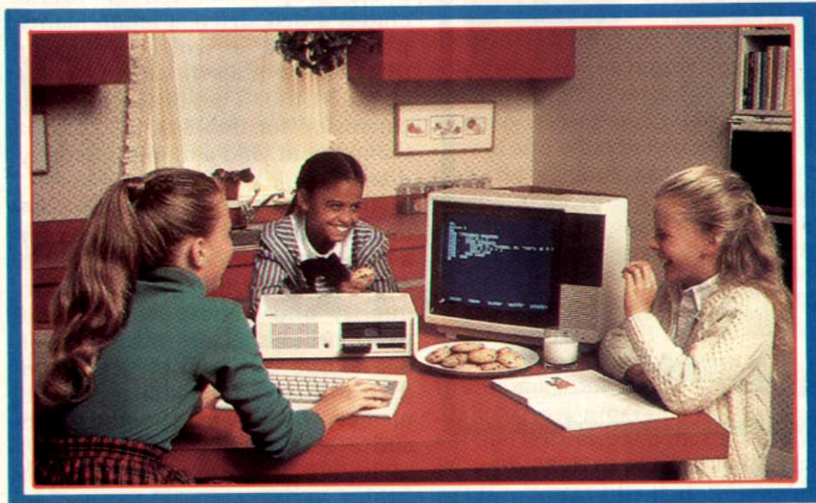
The battery-powered keyboard uses an infrared beam instead of wires.
