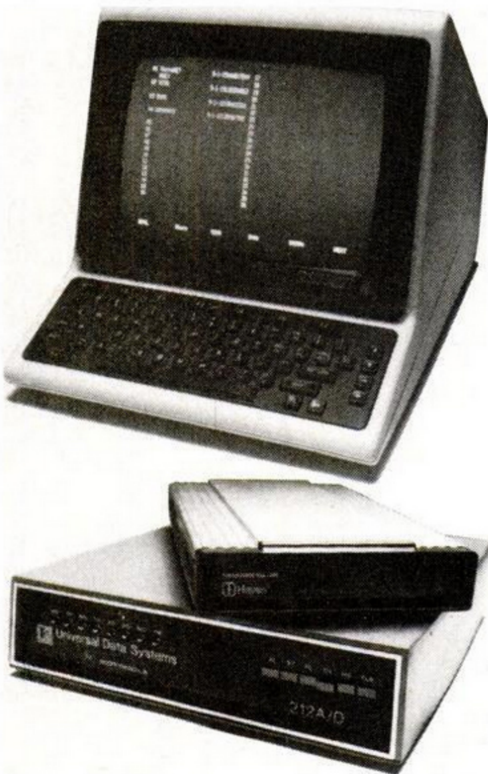
Modems come in various shapes and sizes. Tymshare's Scanset terminal (top) includes both a modem and display with a full keyboard. Hayes Smartmodem 1200 (middle) connects any computer to a phone line. Universal Data System's 212A/D puts a full menu of commands on the connecting computer's screen.
