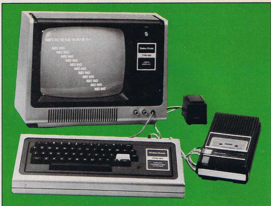
Radio Shack's complete TRS-80 Microcomputer System consists of a 53-key alphanumeric keyboard and microcomputer, 12" video monitor and cassette storage.
