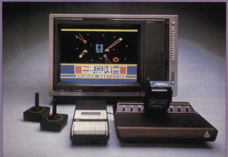
Starpath's Supercharger puts more byte (6,272 of 'em) into the VCS.
