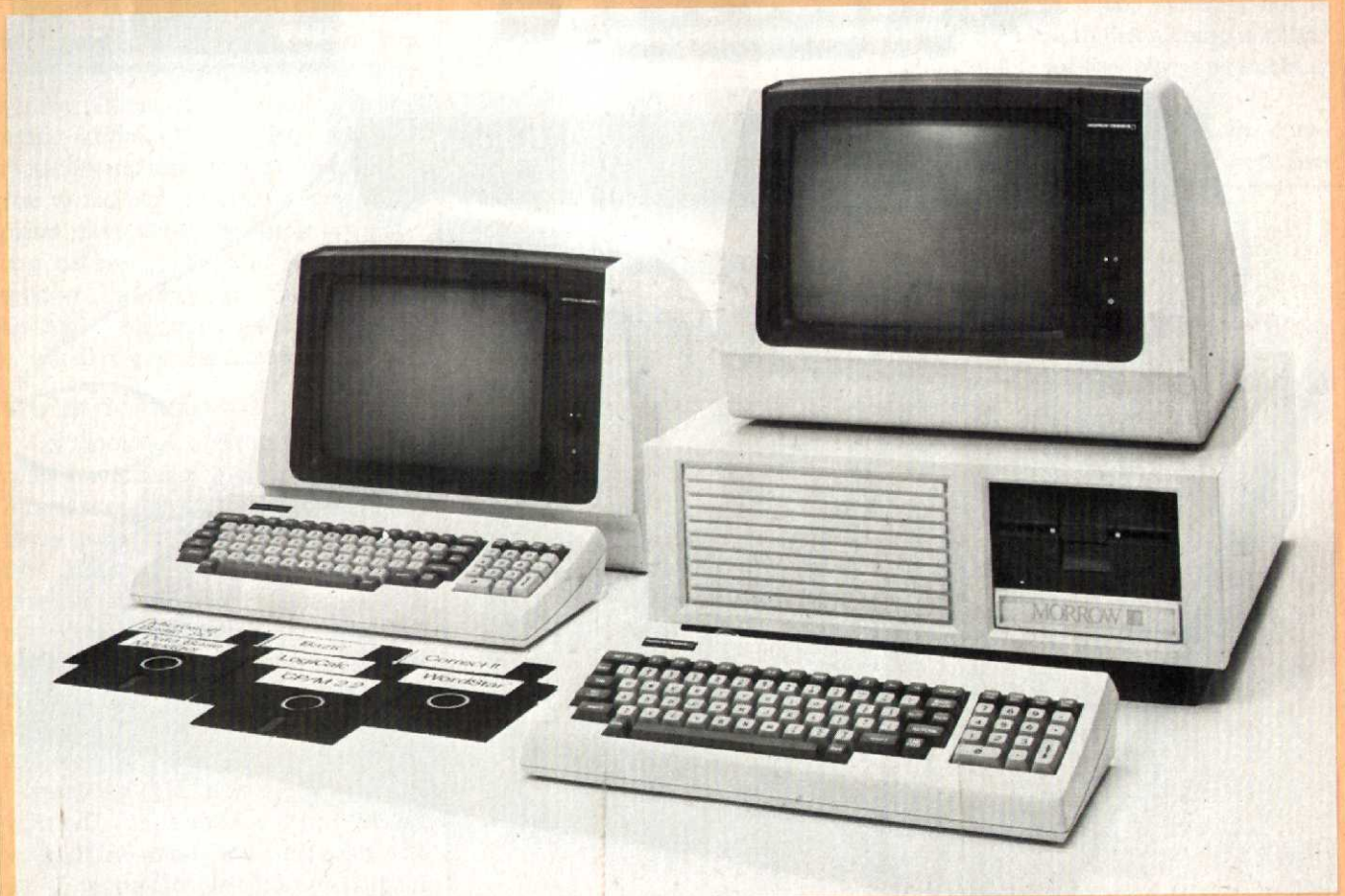
The Morrow Decision I and the expandable S-100 multi-user, multi-tasking computer system.
