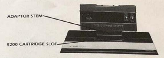
Plug your 2600 controller into the appropriate controller jack on the side of your Adaptor. For one-player games, use the left controller jack; for two-player games, use both controller jacks. (NOTE: Your 5200 controllers will not work with the VCS Cartridge Adaptor.)
