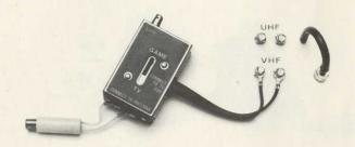
C. Connect the twin-lead wire from the TV/GAME Switch Box to the VHF antenna terminals on your television set.
