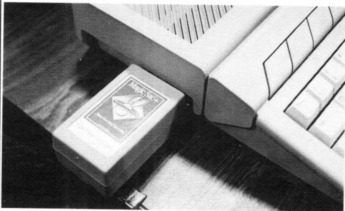
The Magic Sac+ cart that allows an ST to run Mac software.
