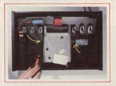
Step 6: Locate the two .22 uf capacitors on the left side of the circuit board as shown. Using a diagonal cutter (wire cutter)—not a scissors—snip the leads going to the capacitors. The unit may now be re-assembled and checked, or you may proceed to replace the capacitors without checking further.
