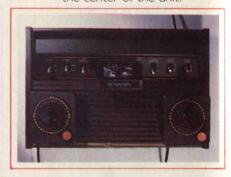
Step 3: Turn unit face up. Ease the cover piece from the base using moderate force by lifting first the rear edge of the cover and then the front. Remove the six black rubber washers
