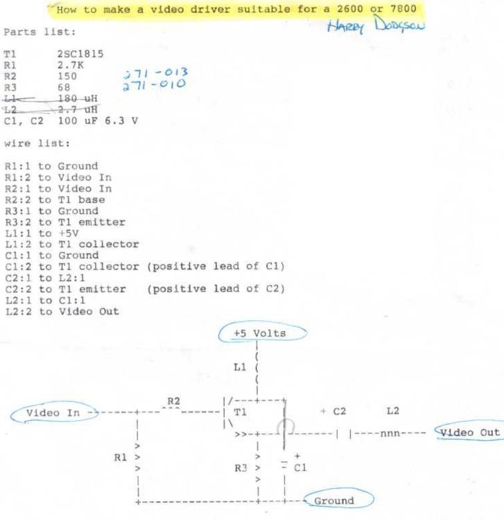
This is a simple common emitter amplifier. It is a non-inverting current amplifier and serves here to allow the video signal from the game to drive a standard composite monitor with 75 ohm impedance.
